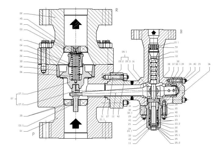
Figure 1 Sectional drawing and parts list of the valve type MRM (example)
