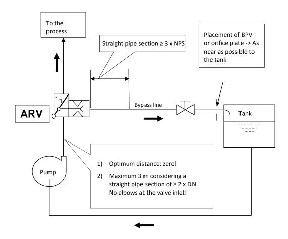
**Figure 10** Schematic representation of the installation conditions for the pump protection valve
