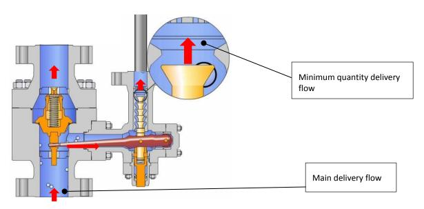
Figure 2 MRM valve with closed non-return plug and open bypass
