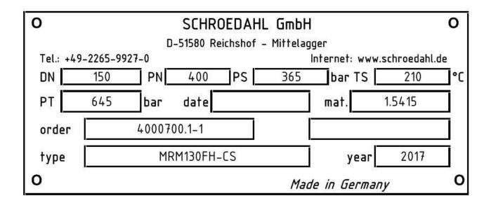
Figure 8 Example of a nameplate of the type MRM
