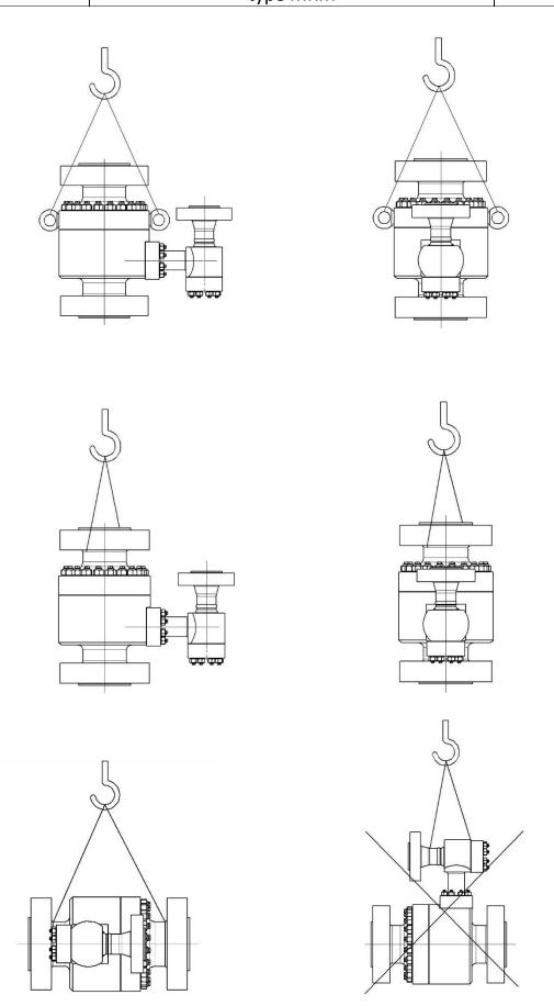
Figure 9 Typical representation of the handling options when installing the valve
